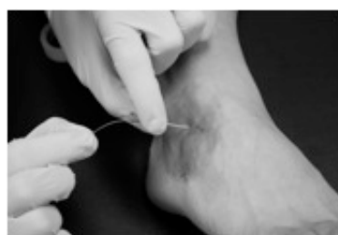
Figure 1: Threading the thermocouple through the inserted catheter.
