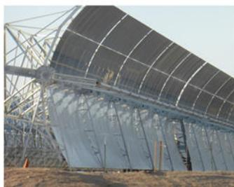
**Figure 2:** The parabolic trough collector. This parabolic trough collector is designed like a parabola. Which may focus the sun at 30 – 100 times the collector's usual intensity.
