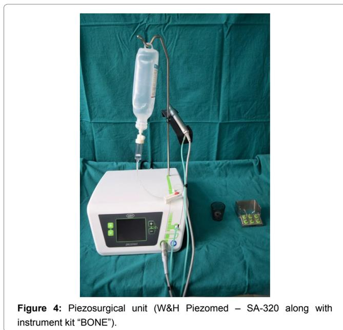
Figure 4: Piezosurgical unit (W&H Piezomed – SA-320) along with instrument kit "BONE".
