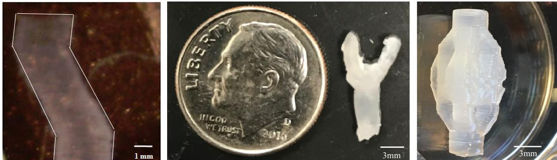
Figure 1: 3D vascular constructs fabricated using different advanced manufacturing technologies: (a) Inkjet printing, (b) Microextrusion and (c) Stereolithography.
