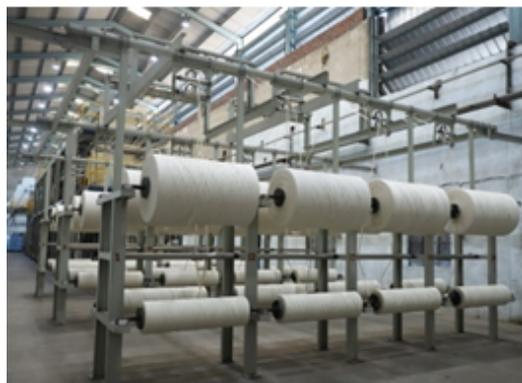
**Figure 5:** Balls at rope dyeing machine.
