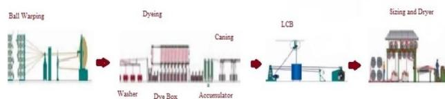
Figure 3: Flow diagram of slasher dyeing and sizing.
