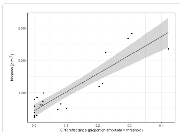
**Figure 5:** Below-ground biomass estimated from GPR returns above a site-specific reflectance level. The model for this data was  $\text{g/m}^3 = 2176.5 + 28664.1 \cdot \text{GPR returns}$ . Adj. R<sup>2</sup> .79, p
