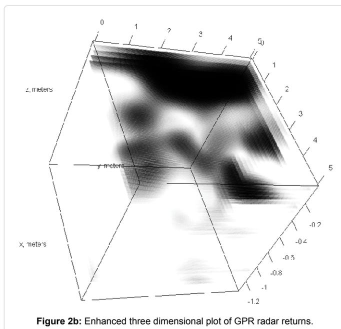
Figure 2b: Enhanced three dimensional plot of GPR radar returns.
