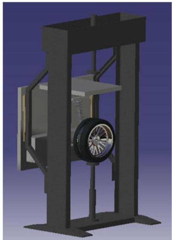
Figure 4: Fully assembled model of suspension test rig.
