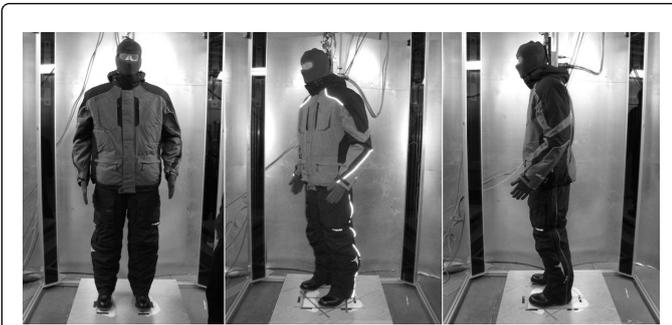
**Figure 2:** Effects of wind direction (wind speed 8 m/s) on effective thermal insulation ( $I_{cle}$ ) of clothing ensemble C3, tested at angles of 0°, 45° and 90° to the wind.
