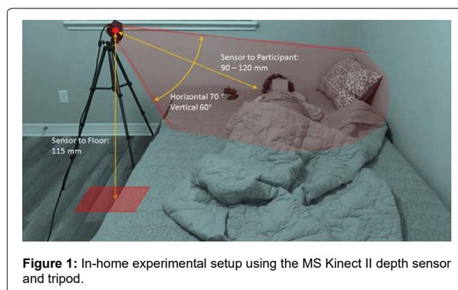
Figure 1: In-home experimental setup using the MS Kinect II depth sensor and tripod.
