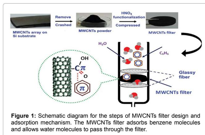
**Figure 1:** Schematic diagram for the steps of MWCNTs filter design and adsorption mechanism. The MWCNTs filter adsorbs benzene molecules and allows water molecules to pass through the filter.
