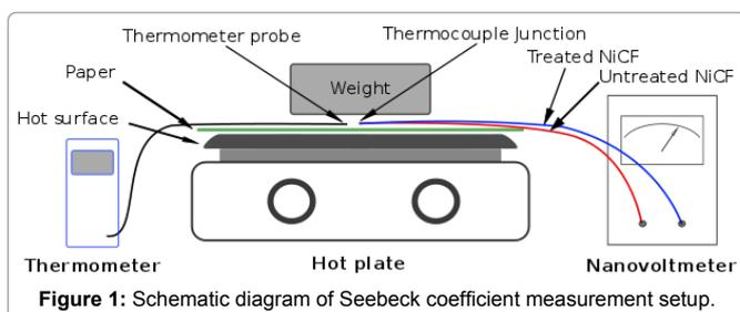
Figure 1: Schematic diagram of Seebeck coefficient measurement setup.
