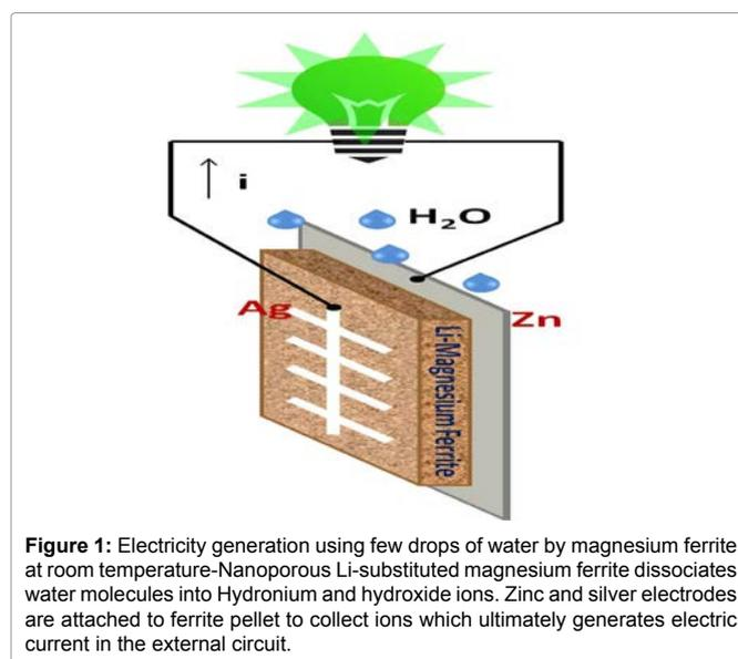
**Figure 1:** Electricity generation using few drops of water by magnesium ferrite at room temperature-Nanoporous Li-substituted magnesium ferrite dissociates water molecules into Hydronium and hydroxide ions. Zinc and silver electrodes are attached to ferrite pellet to collect ions which ultimately generates electric current in the external circuit.
