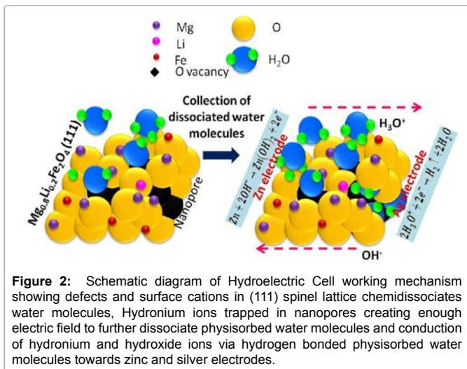
generation methods compared to photo-biosynthesis, photo-electrocatalysis and thermo-chemical methods etc. High purity hydrogen gas is produced by applying external voltage on hydroelectric cell.
