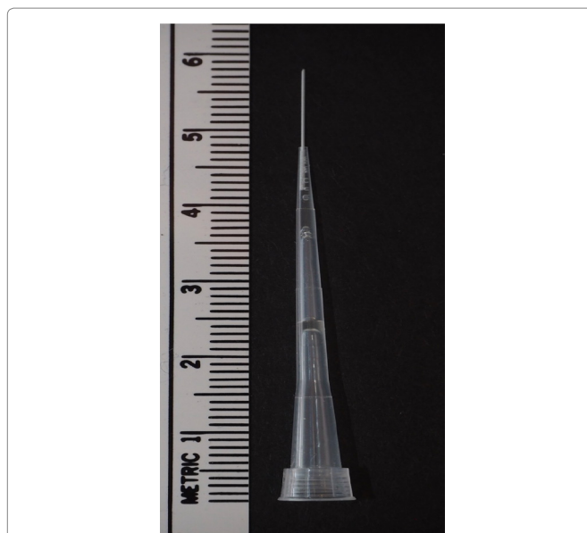
Figure 1: Biocompatible Solid-Phase Microextraction (BioSPME) fiber tippet.
