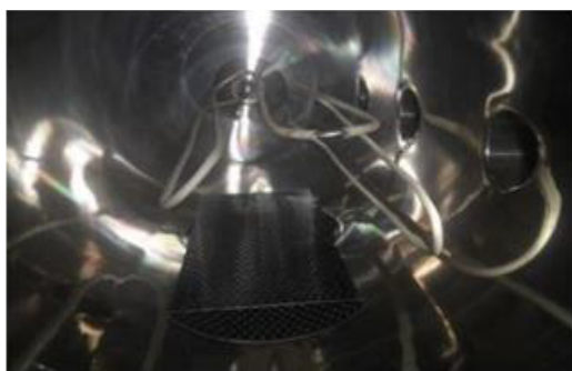
Figure 4: Helical antenna inside the vacuum tube.
