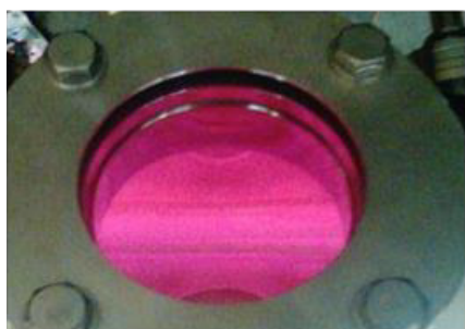
Figure 5: Plasma generation inside the vacuum chamber.
