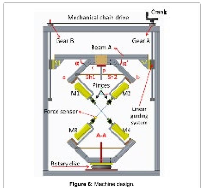
Figure 6: Machine design.
