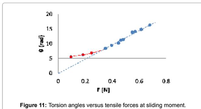
Figure 11: Torsion angles versus tensile forces at sliding moment.
