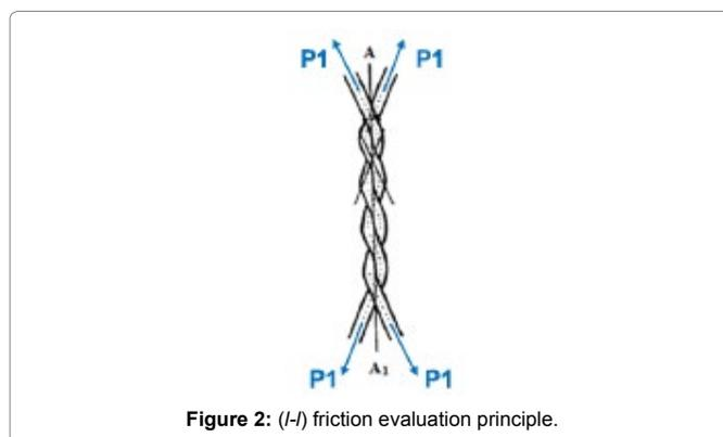
Figure 2: (l-l) friction evaluation principle.
