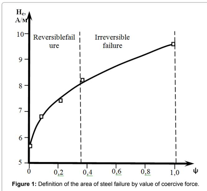
Figure 1: Definition of the area of steel failure by value of coercive force.
