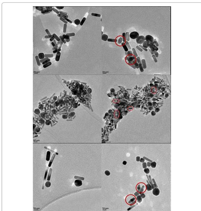
**Figure 3:** TEM images of AuNRs having LP peaks at 696 nm (top), 770 nm (middle) and 910 nm (bottom), before (left) and after (right) completion of all laser irradiation steps described in the text. Red circles show the partially melted, and hence deformed,  $\Phi$ -shaped particles.
