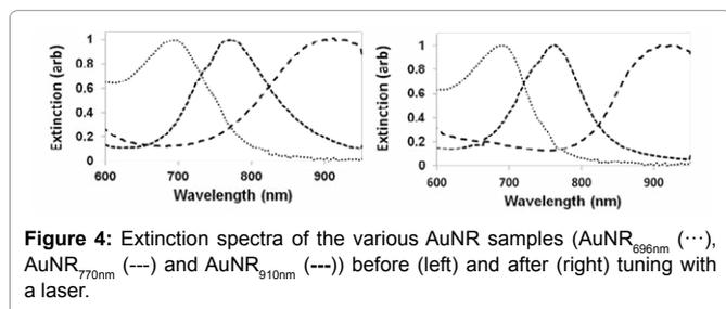
**Figure 4:** Extinction spectra of the various AuNR samples (AuNR<sub>696nm</sub> (···), AuNR<sub>770nm</sub> (---) and AuNR<sub>910nm</sub> (-·-·)) before (left) and after (right) tuning with a laser.
