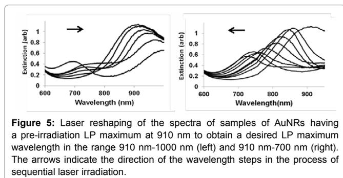
**Figure 5:** Laser reshaping of the spectra of samples of AuNRs having a pre-irradiation LP maximum at 910 nm to obtain a desired LP maximum wavelength in the range 910 nm-1000 nm (left) and 910 nm-700 nm (right). The arrows indicate the direction of the wavelength steps in the process of sequential laser irradiation.
