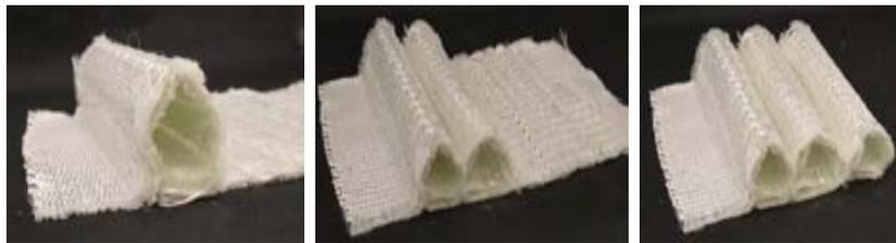
Figure 7: Realization of PACS by folding a woven layer consisting of compliant sections and flank sections with inserts.
