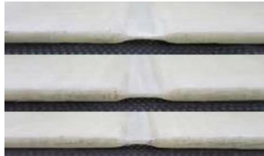
Figure 6: Weaving of compliant and flank sections of PACS using hybrid yarns and consolidated compliant mechanism.
