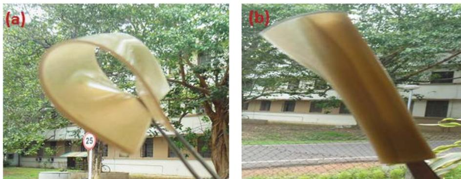
Figure 11: Flexibility study of EMA/SP composite (EMSP-10) at 2 mm thickness, (a) bent and (b) rolled state.
