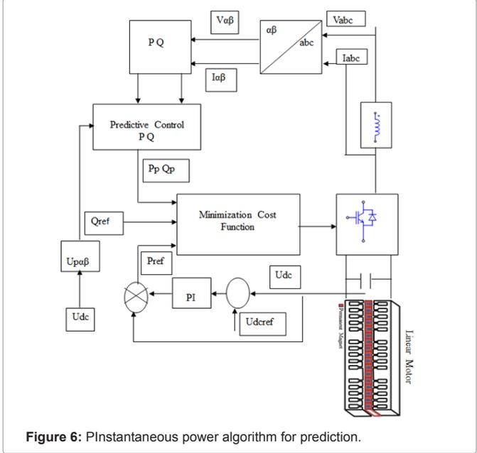
Figure 6: PInstantaneous power algorithm for prediction.
