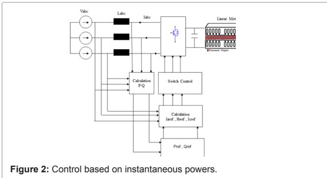
Figure 2: Control based on instantaneous powers.
