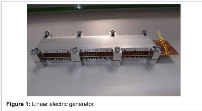
Figure 1: Linear electric generator.
