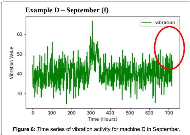
can be established. Therefore, the RUL will still be calculated, but the term TTF will be used to replace the concept of the RUL. Both serve the same purpose, but TTF more accurately describes the situation of identifying vibration-related failures with no performance related metrics considered. The pattern of which vibration escalates needs to be identified and calculated to be able to predict vibration-related failures instead.
