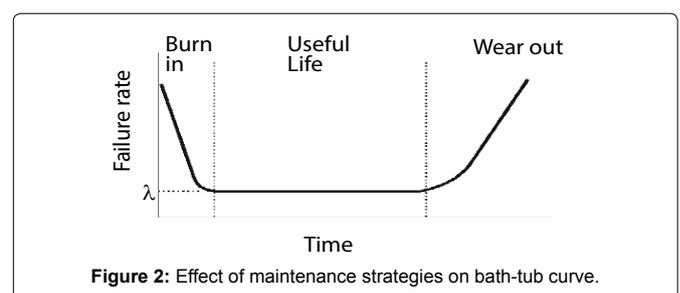
Figure 2: Effect of maintenance strategies on bath-tub curve.
