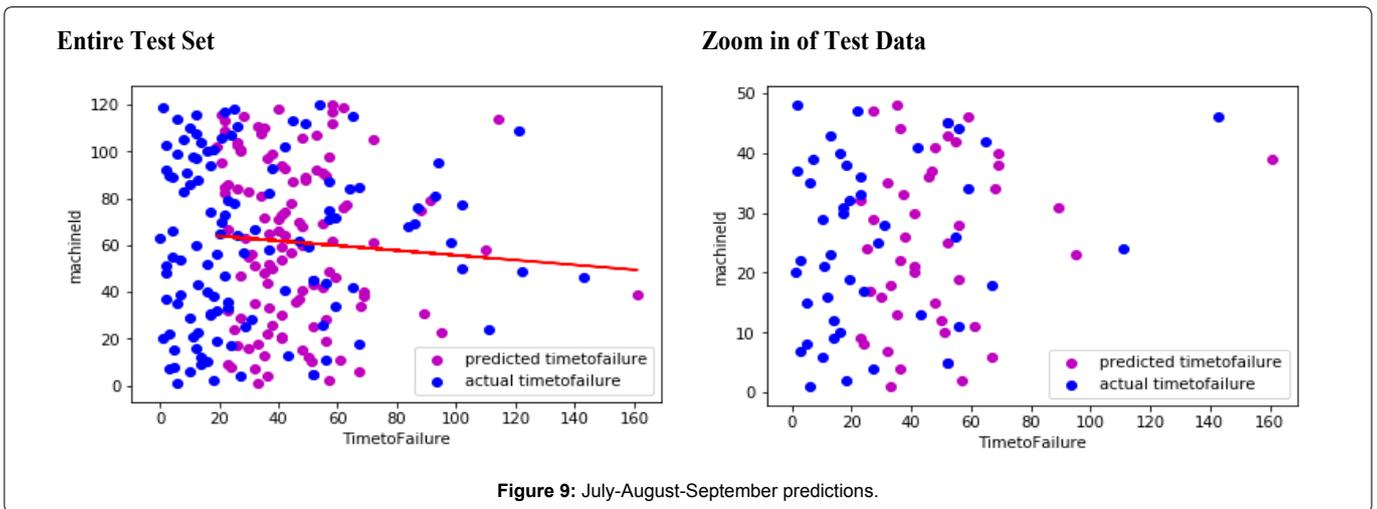
predictions made by the algorithm, the overall accuracy over the four tests is underwhelming at best. Within its current state, the prototype would not be suitable as a predictive maintenance solution, as it is completely transparent that the prototype requires additional work outside the project plan.
