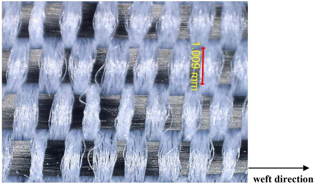
Figure 1: The view on a single layer of a woven structure made of polyester warps and carbon wefts.
