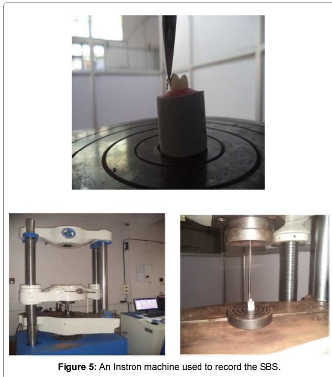
Figure 5: An Instron machine used to record the SBS.
