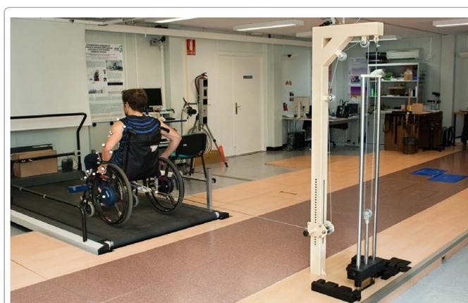
Figure 1: Overview of the test set-up where the subject is working against extra resistance applied through a pulley system and in which the positions of the markers are shown.
