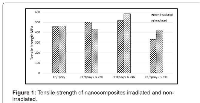
Figure 1: Tensile strength of nanocomposites irradiated and non-irradiated.
