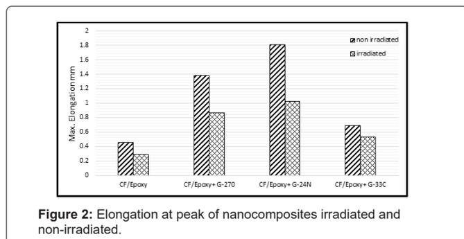
Figure 2: Elongation at peak of nanocomposites irradiated and non-irradiated.
