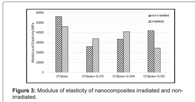
Figure 3: Modulus of elasticity of nanocomposites irradiated and non-irradiated.
