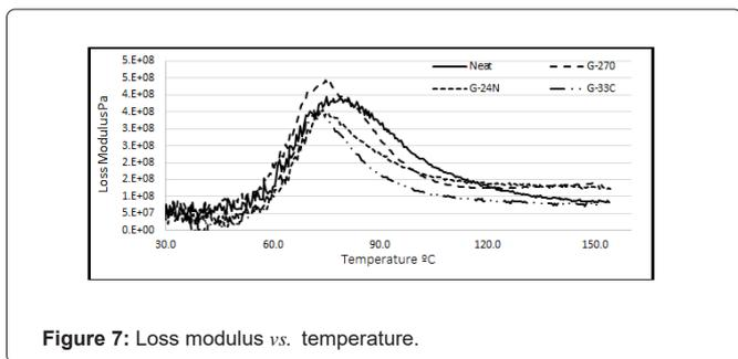
Figure 7: Loss modulus vs. temperature.
