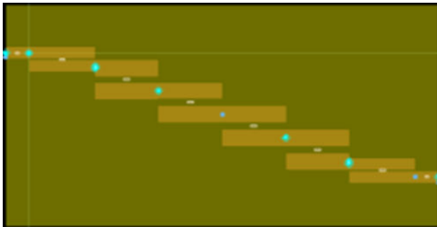
Figure 9: Layout of BPF with 75.08 mm × 39 mm ground plane.
