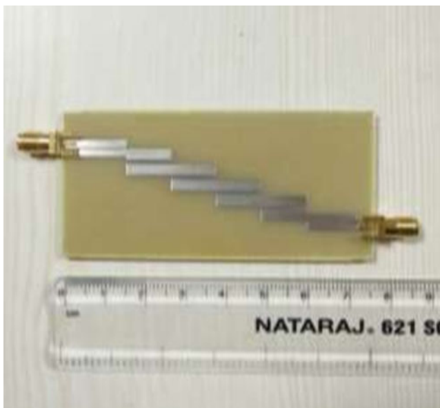
Figure 11: Photograph of fabricated coupled line BPF.
