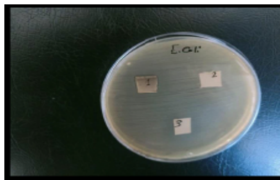
Figure 14: The Effect of treated fabrics against Gram-negative ( Escherichia coli ).
