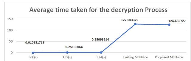
Figure 10: Average time taken for the decryption process of various algorithms.
