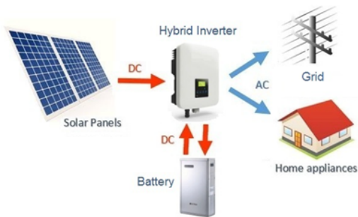
Figure 3: illustrates the hybrid system for electricity generation by using solar and grid power.
