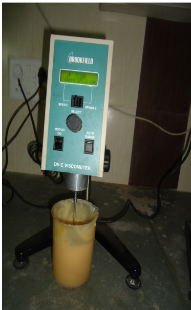
Figure 3: DV-e rotational brook field viscometer.
