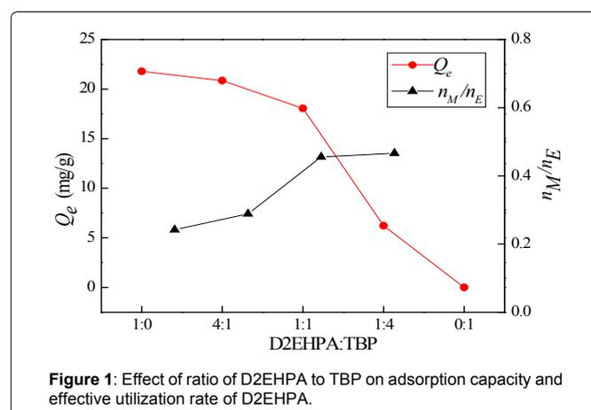
Figure 1: Effect of ratio of D2EHPA to TBP on adsorption capacity and effective utilization rate of D2EHPA.
