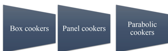
Figure 4: Schematic representation of the classification of the solar cookers based on the configuration.
