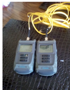
Figure 6: Laser source and power meter used in attenuation measurements.
