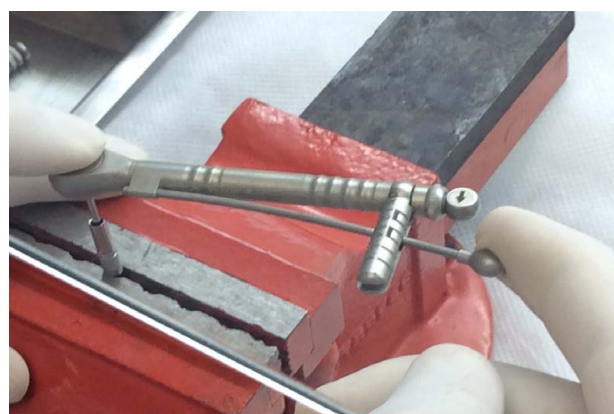
Figure 2: Application of the torque recommended by the manufacturer to the screw of the prosthetic abutment.
