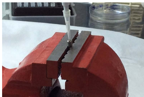
Figure 1: Solution containing Escherichia coli that was inoculated into the internal part of the implant.
