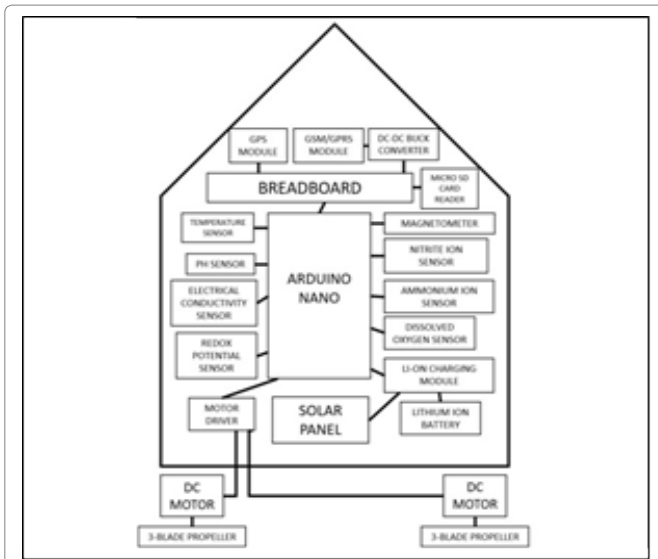
Figure 2: Block diagram Representation of System Chassis and Component arrangement.
