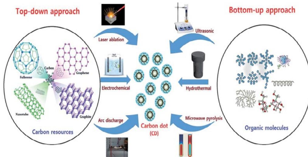
Figure 2: Different approaches to synthesize carbon dots.
