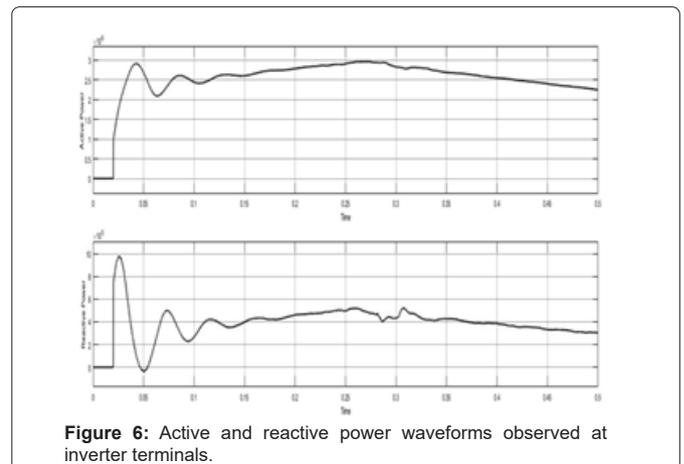
**Figure 6:** Active and reactive power waveforms observed at inverter terminals.
