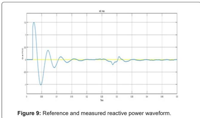
Figure 9: Reference and measured reactive power waveform.
