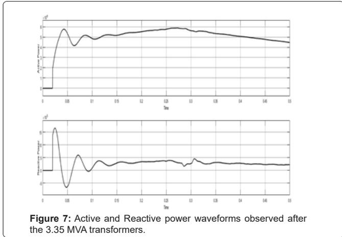
Figure 7: Active and Reactive power waveforms observed after the 3.35 MVA transformers.
