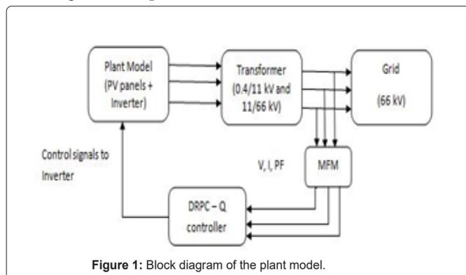
Figure 1: Block diagram of the plant model.
