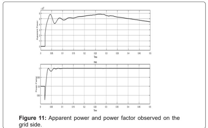
Figure 11: Apparent power and power factor observed on the grid side.
