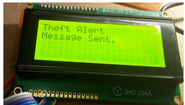
Figure 8: LCD displaying alert in case of shorting the phase.
