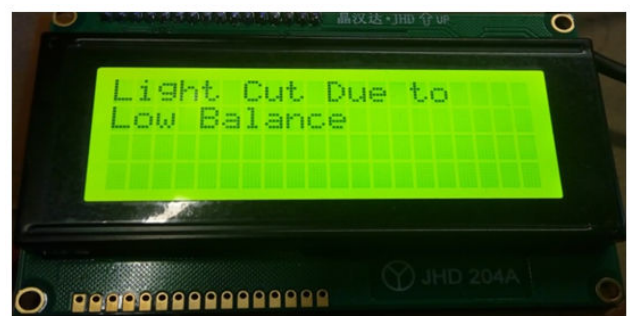
Figure 9: LCD displaying message in case of power cut due to low balance.
