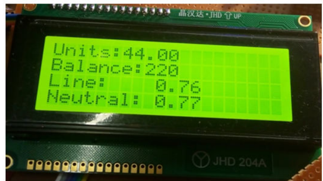
Figure 7: LCD displaying balance and the units consumed.
