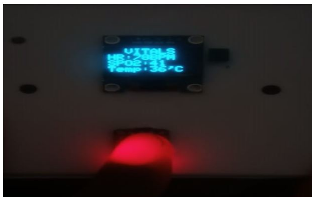
Figure 5d: Touching the OLED screen displays the user's vitals.
