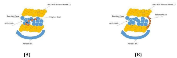
Figure 1: Schematic of DPD particle motion in a channel. (A) Free motion, (B) Resisted motion.
