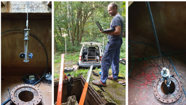
Figure 2: Left: Lowering the ultrasonic emitter into the borehole; Middle: The device in process with an operator using a laptop to control the system; Right: The probe after re-emerging from the borehole.
