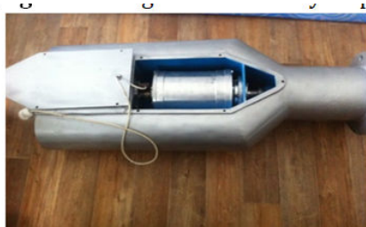
Figure 9: Micro hydropower plant.
