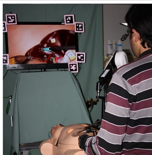
Figure 1: Experimental study setup: OR phantom ELITE (CLA, Coburg, Germany), SOLOASSIST robotic camera control (AKTORMed, Barbing, Germany), color-marked laparoscopic instrument and head-mounted eye-tracking system (Ergoneers, Geretsried, Germany).
