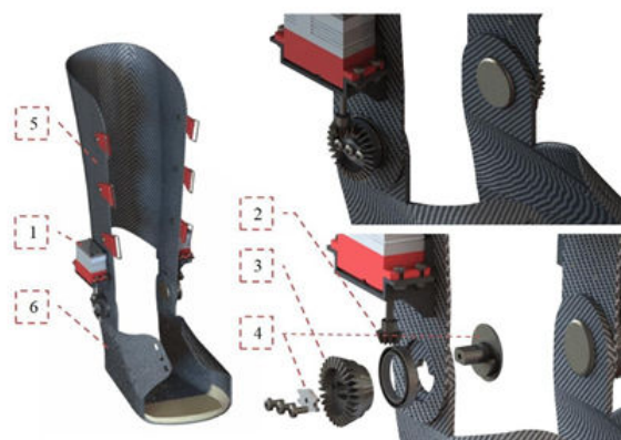
Figure 6: Assembly of the ExoGaitOR. 1: servo motor, 2: pinion gear, 3: gear, 4: connection part, 5: upper orthosis part, 6: lower orthosis part.
