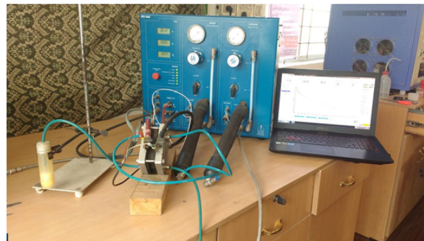
Figure 7: Bio-logic FCT fuel cell test station used for performance evaluation.
