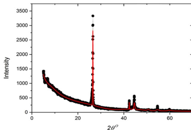
**Figure 3:** Comparison between experimental (black dots) simulated XRD patterns obtained for graphite sample. Note: ● Experimental — Simulated
