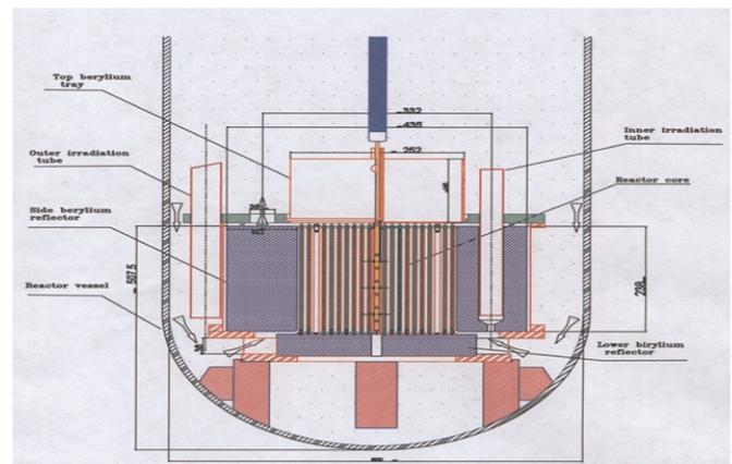
**Figure 1:** Location of inner and outer irradiation sites of the MNSR reactor.
