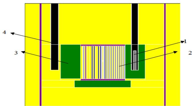
Figure 8: Vertical cross section of MNSR by MCNP4C code, where: 1-IIT with chain of TPCC filled with reflector material, 2-fuel, 3-Be reflector, 4-outer irradiation site.
