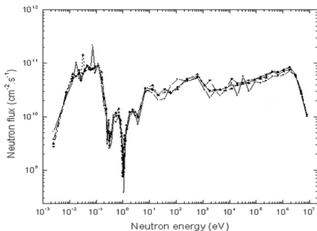
Figure 9: The neutron flux for 69 energy groups in the IIT of the MNSR reactor with chains of the potential reflectors (H<sub>2</sub>O, D<sub>2</sub>O and Gr).
