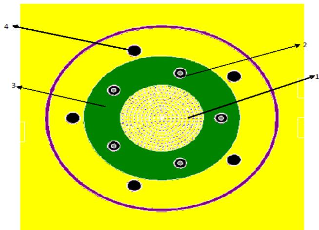
Figure 7: Horizontal cross section of MNSR by MCNP4C code, where: 1-inner irradiation site with chain of TPCC filled with reflector material, 2-fuel, 3-Be reflector, 4-outer irradiation site.
