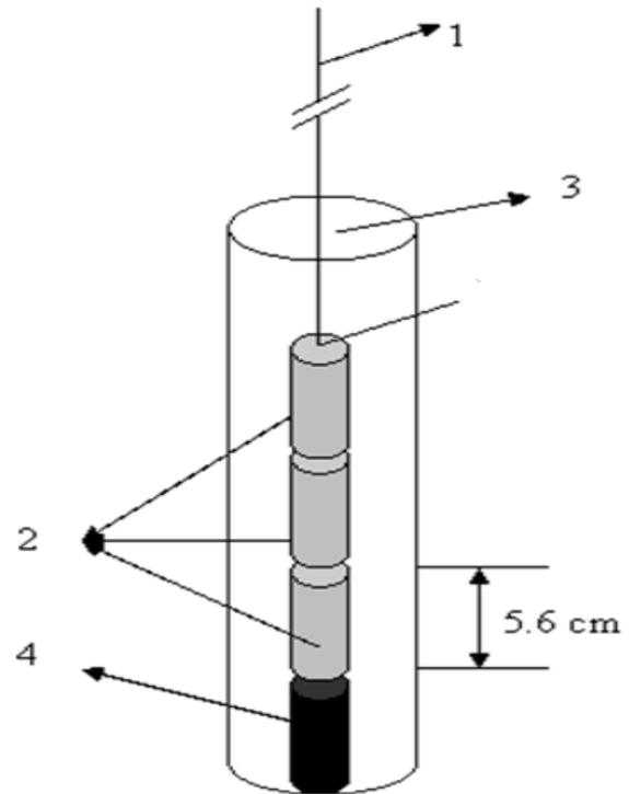
**Figure 6:** IIT filled with reflector material, where: 1-long rope, 2-a chain of TPCC filled with reflector material, 3-IIT, 4-irradiation capsule. Note:  $\Phi=1.45$  cm
