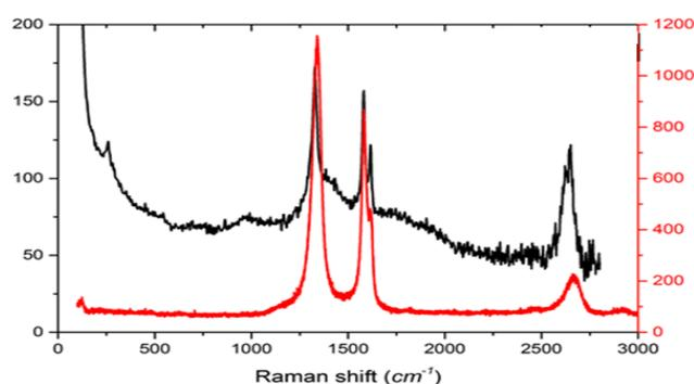
**Figure 4:** Comparison between experimental (red line) and black line) Raman spectra of graphite. Note: — Reference — Sample
