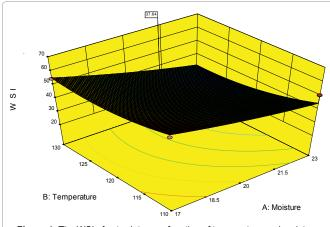
Figure 4: The WSI of extrudate as a function of temperature and moisture at optimized screw speed (375 rpm). Note: WSI: Water solubility index.
