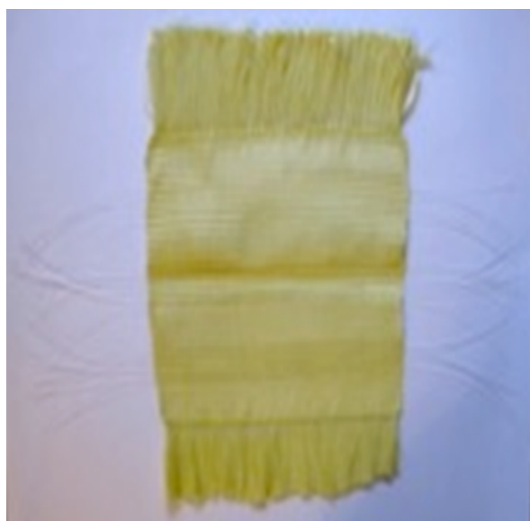
Figure 2l: Smart dining tablecloth sample 12 (check weave/flame retardant polyester yarn and optical fiber).
