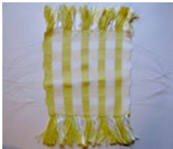
Figure 2h: Smart dining tablecloth sample 8 (basket weave/100% polyester yarn, 100% cotton yarn, and optical fiber).
