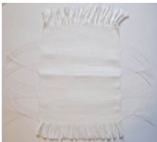
Figure 2g: Smart dining tablecloth sample 7 (plain weave/100% polyester yarn, 100% cotton yarn, and optical fiber).
