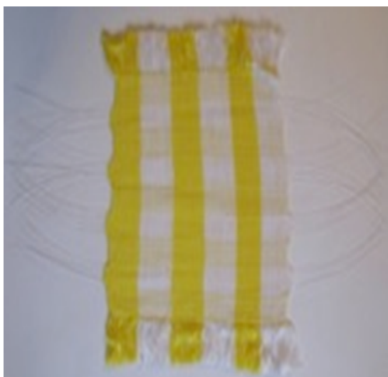
Figure 2f: Smart dining tablecloth sample 6 (check weave/100% cotton yarn and optical fiber).
