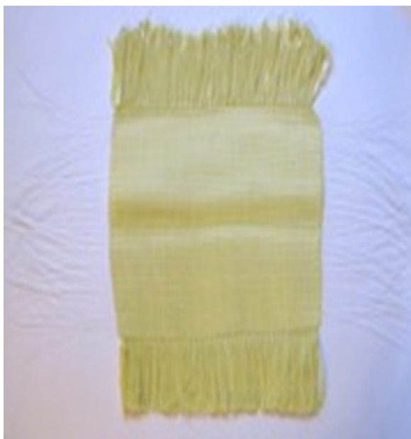
Figure 2k: Smart dining tablecloth sample 11 (basket weave/flame retardant polyester yarn and optical fiber).
