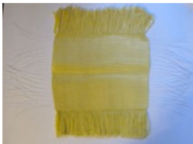
Figure 2j: Smart dining tablecloth sample 10 (plain weave/flame retardant polyester yarn and optical fiber).
