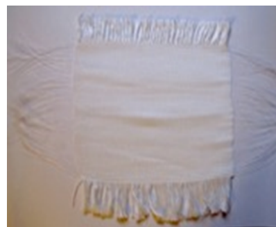
Figure 2a: Smart dining tablecloth sample 1 (plain weave/100% polyester yarn and optical fiber)
