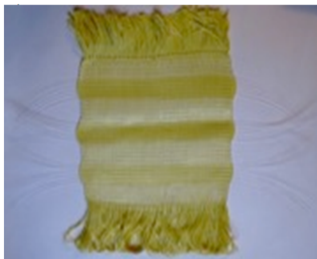
Figure 2i: Smart dining tablecloth sample 9 (check weave/100% polyester yarn, 100% cotton yarn, and optical fiber).
