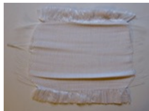
Figure 2d: Smart dining tablecloth sample 4 (plain weave/100% cotton yarn and optical fiber).
