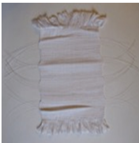
Figure 2e: Smart dining tablecloth sample 5 (basket weave/100% cotton yarn and optical fiber).
