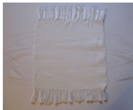
Figure 2b: Smart dining tablecloth sample 2 (basket weave/100% polyester yarn and optical fiber).
