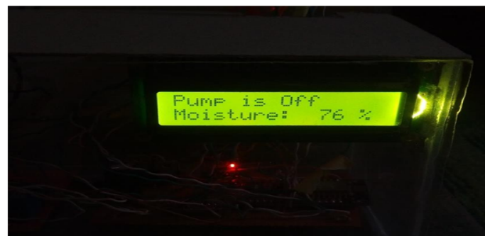
Figure 14: Soil moisture at 76% (pump off).
