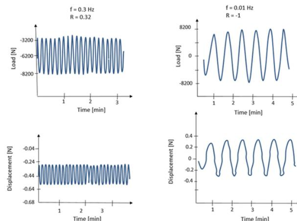
Figure 9: Displacement and load curves as a function of time (f=0.3 Hz, R=0.32 and f=0.01 Hz, R=-1).
