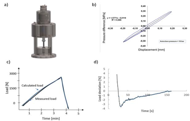
Figure 6: Intrinsic stiffness of the DB loading apparatus at 23°C.
