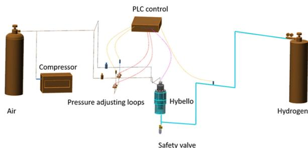
Figure 8: Layout for the Hybello material testing device setup.
