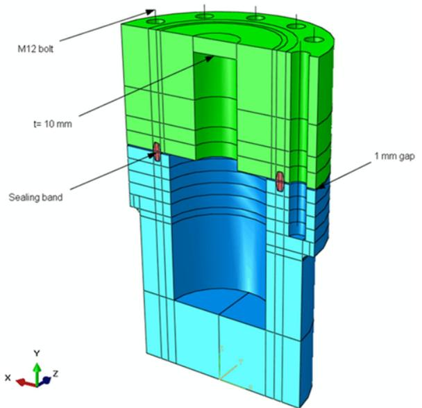
Figure 2: Structure of the pressure vessel.
