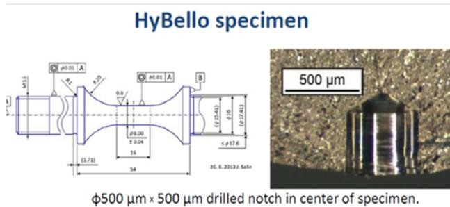
**Figure 10:** An illustration to show the location and type of small drilled hole used in the research. The measurements are given in mm unless marked as  $\mu\text{m}$ .
