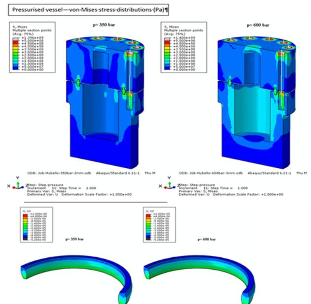
Figure 3: The stress distribution on the structure.
