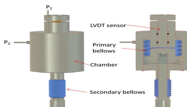
**Figure 4:** The DB loading apparatus.
