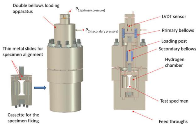
Figure 1: The main structure of the Hybello.
