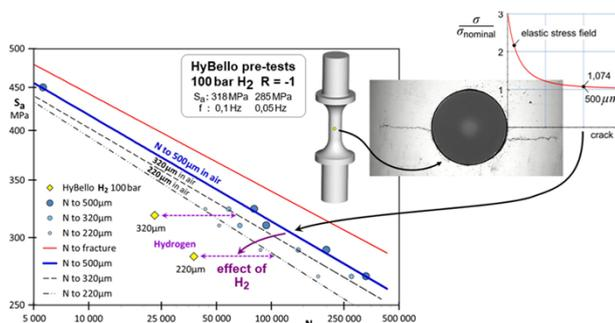
**Figure 11:** The results of the fatigue tests performed in the Hybello.
