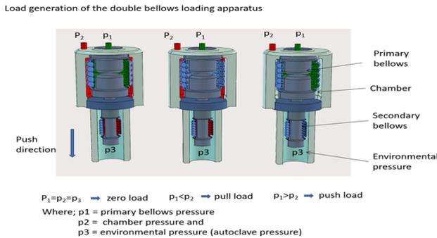
Figure 5: Load generation of the DB loading apparatus.
